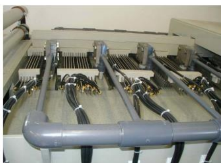
2. step: electrochemical de-colouration
