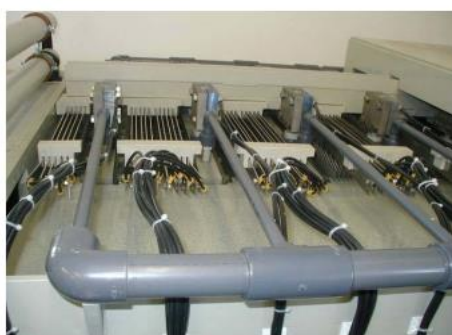
2. step: electrochemical de-colouration
