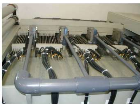
2. step: electrochemical de-colouration
